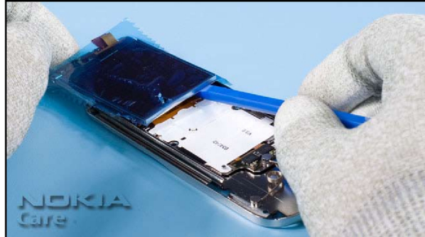
26. Start lifting up the glued in LCD at the shown side first.
